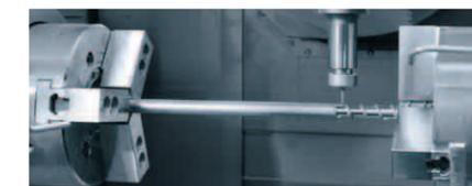
The second spindle of the INTEGREX draws out the workpiece to the programmed length to achieve shorter machining time and high-precision screw machining
