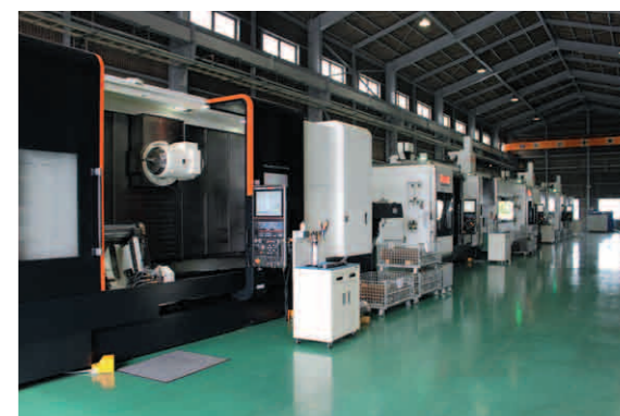
Machining area composed of the INTEGREGX series to process main components of the GUZZILLA
