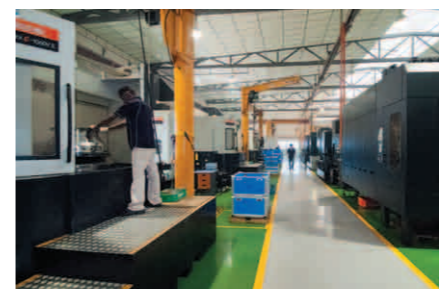
Horizontal machining center MEGA 8800 and large multi-tasking machine INTEGREX e-1060V/6 II are installed along with other machines
