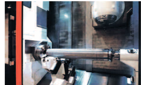
INTEGREX e-500H II machines rolls in a single machine setup
