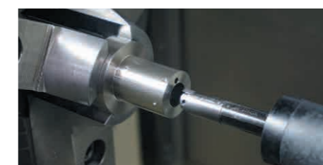
Housing of a touch probe machined with the INTEGREX
