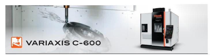
The VARIAXIS C-600, simultaneous 5-axis vertical machining center is designed to be easily integrated with automation systems thanks to the flat surface of the front of the machine and the large operation area. The front door and right side door can be automatically opened/closed for workpiece loading/unloading by a robot.
