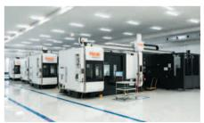
FMS line of the INTEGREX i series installed in Sankyo Dream Factory
