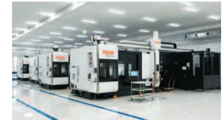
FMS line of the INTEGREX i series installed in Sankyo Dream Factory
