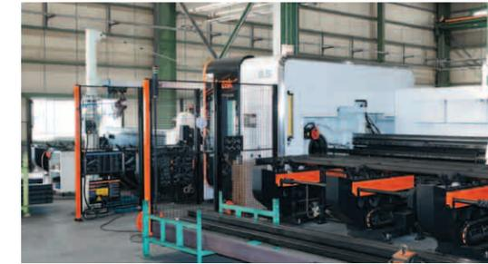
3D FABRI GEAR 220 II is used for 3D cutting of steel tubes
