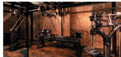
In the "Line shaft drive factory" area, which exhibits belt driven lathes, milling machines, etc., a plant of more than 100 years ago has been reproduced so that visitors can learn what manufacturing was like at that time.
