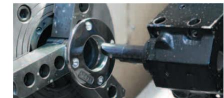
Finish machining of the inside of a lost-wax casting component
