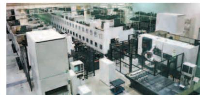
Metal parts of machine tools are produced in the automatic machining plant (Mazak iSMART Factory™). Visitors can see a modern plant using advanced technologies including IoT and automated robots.
