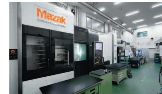
Machining of complex parts with multi-tasking machines is the strength of the company
