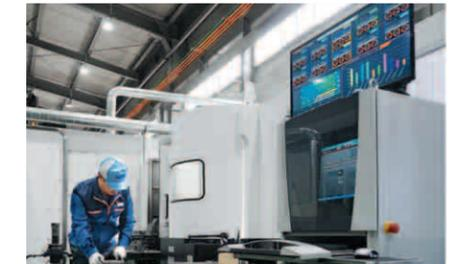
Smooth Monitor AX monitor (upper right in picture) facilitates sharing of equipment operation status
