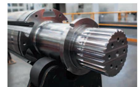
Spline and slotting detail on FLSmidth ABON Sizer Shaft
