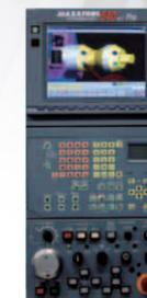
CNC system developed by incorporating the concept of "integration of CNC and PC." This made it possible for machine tools to be easily integrated in a factory network for convenient production management including control of machining programs and tool data.
