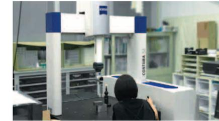
Coordinate measuring machine was introduced to guarantee high precision
