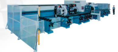
First 3D FABRI GEAR laser processing machine – automatic 5-axis cutting of long pipe and structural material. High accuracy cutting of the complex contours required for tight pipe joints significantly reduced the time required for processing structural material.
