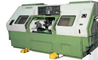
First MULTIPLEX turning center - a single machine with the machining capacity equivalent to that of two CNC lathes. This innovative two-turret/two-spindle design drew much attention from manufacturers worldwide.
