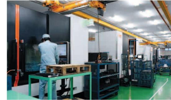
High-speed and high-precision machining with Mazak vertical machining centers
