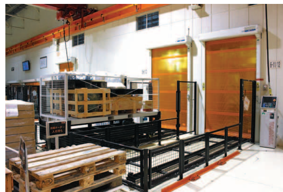
Large parts being input to high-speed automatic vertical stockers
