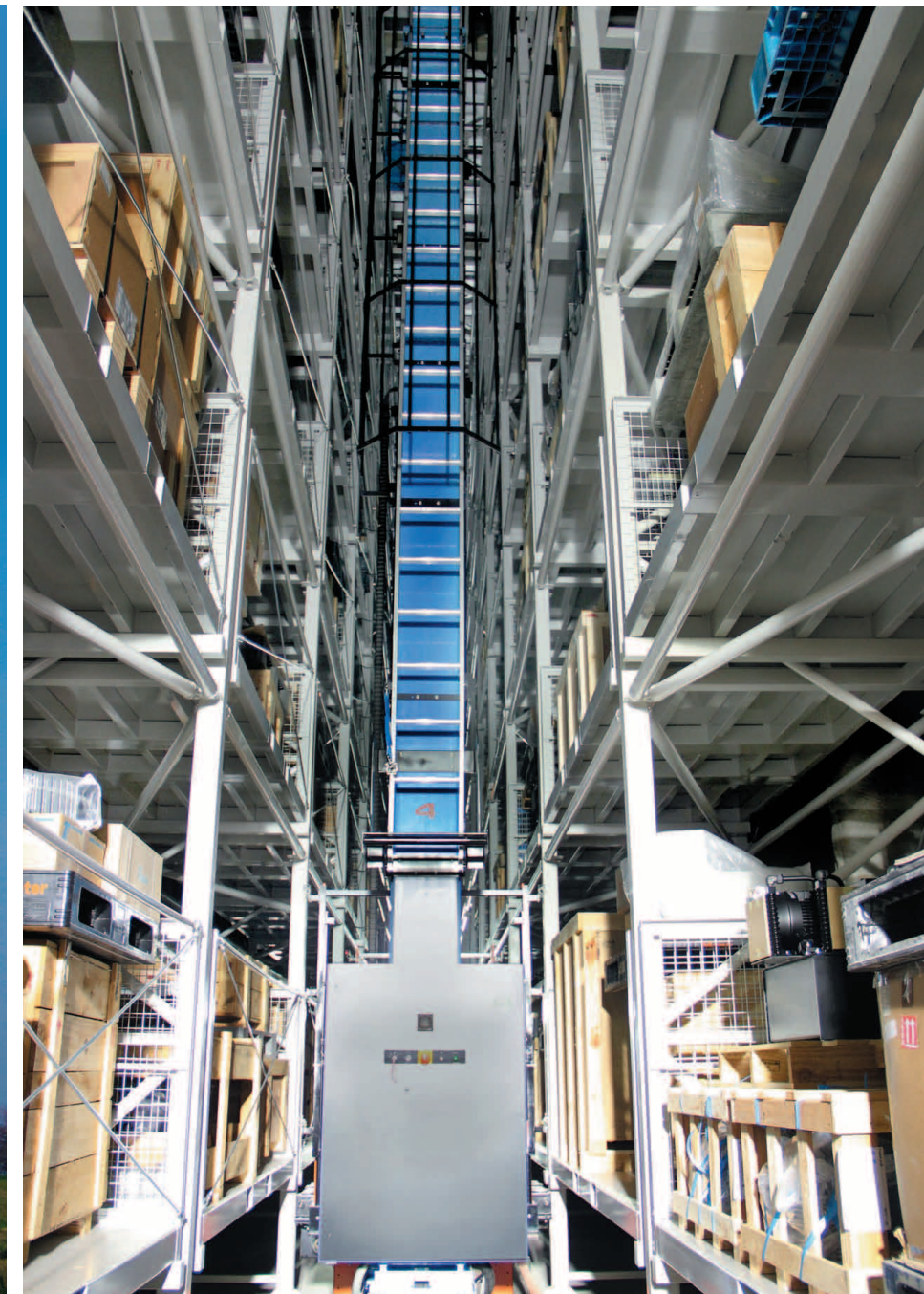
Vertical stocker cranes for medium to large-size parts and a high-speed vertical automatic stocker for small parts
