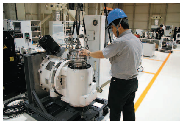
Milling spindle cartridge on test stand
