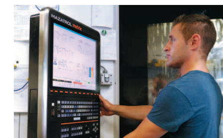
Operator programming a MAZATROL CNC
