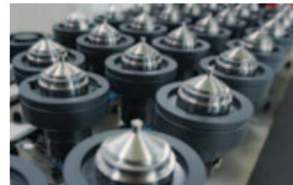
Hot runner nozzles machined by a QUICK TURN SMART
