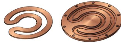
A backing plate is a component of a film deposition system used in the process to manufacture semiconductors, liquid crystal panels and other products. It serves to hold target materials\* in a vacuum chamber (a container to create a vacuum environment). The plate has a water channel because the target materials become high temperature by chemical reactions.
